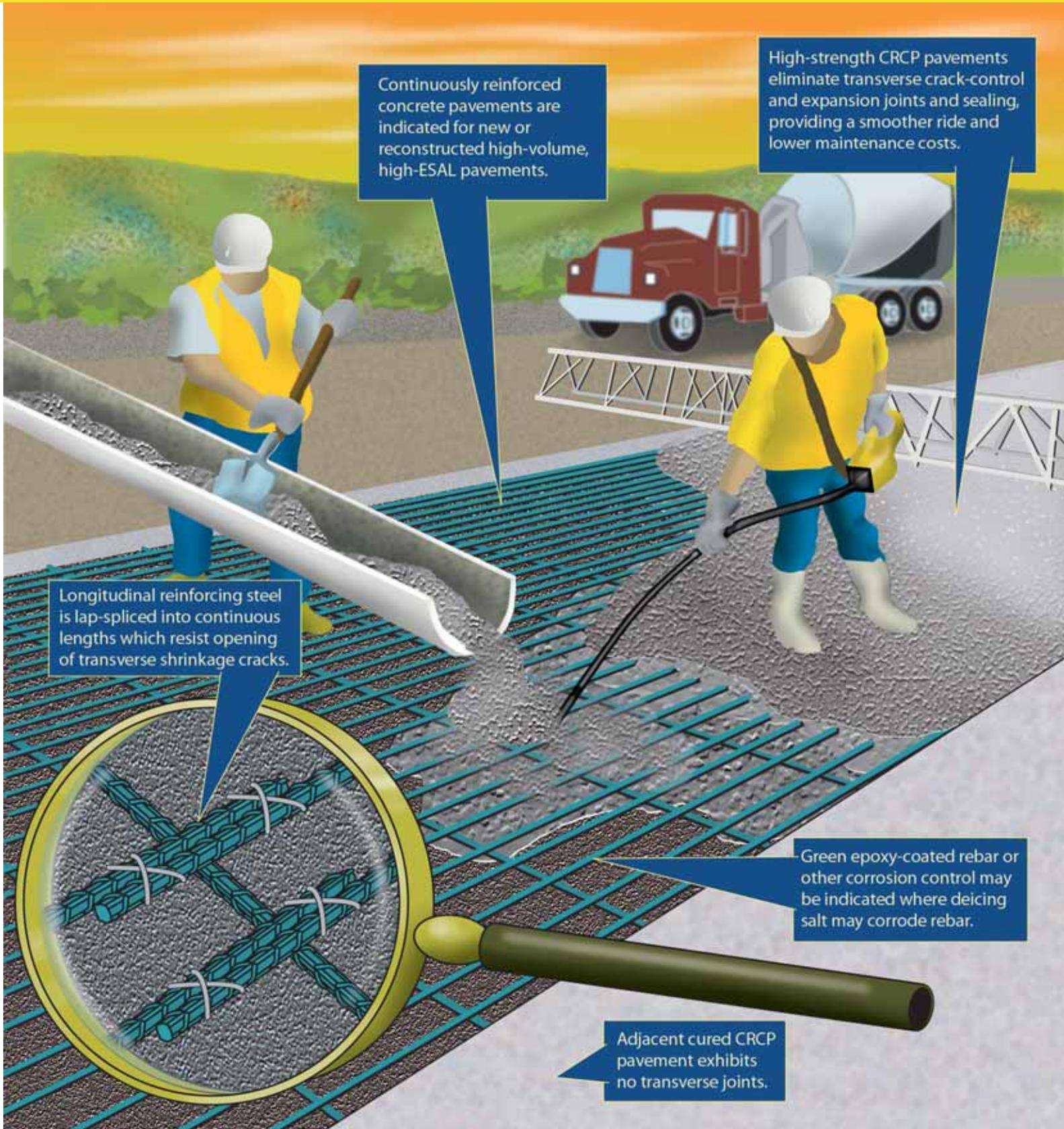
Continuously reinforced concrete pavements are indicated for new or reconstructed high-volume, high-ESAL pavements.
