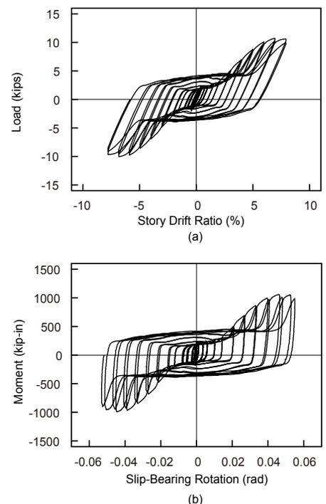
Figure 4: Typical Hysteresis Response: (a) Overall Response; (b) Bolted Moment Connection Component.
