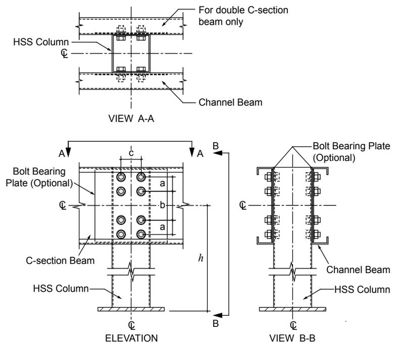
Figure 2: Typical CFS-SBMF Moment Connection.
