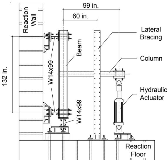
Figure 3: Test Setup.
