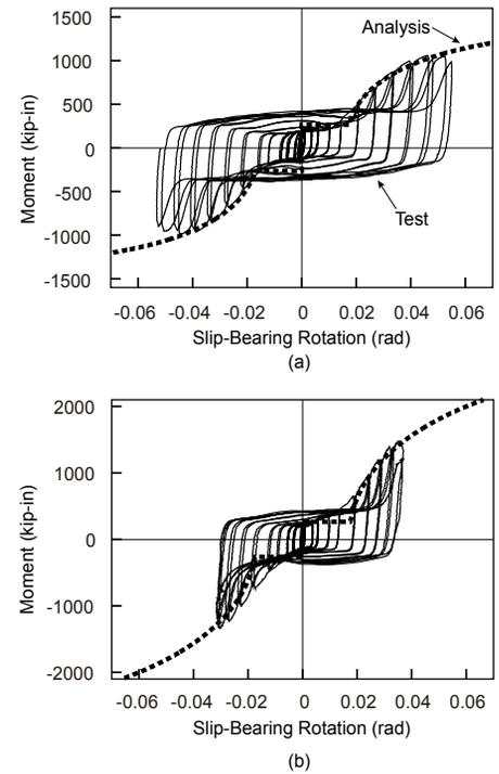
Figure 6: Measured versus Predicted Responses: (a) Specimen 3; (b) Specimen 4.
