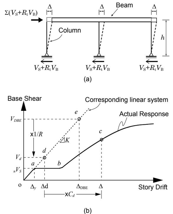
Figure 7: CBF-SBMF Expected Response: (a) Yield Mechanism and Column Shear Distribution; (b) General Structural Response.
