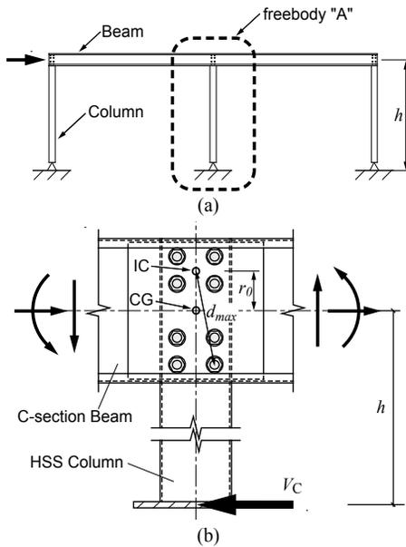
Figure 5: Bolt Group in Eccentric Shear: (a) CFS-SBMF; (b) Freebody "A".
