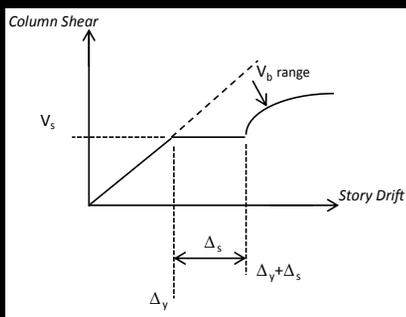
Figure 2: Structural Response of Bolted Connection.
