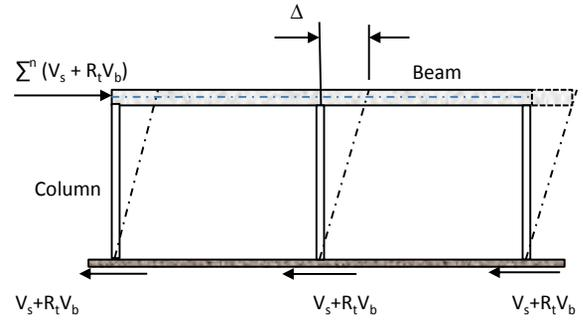
Figure 3: Column Vase Shear.
