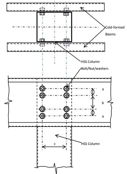
Figure 1: Bolted Connection-SBMF
