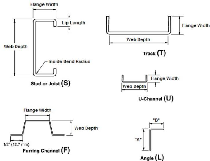
**Figure 4: Cold Formed Steel Framing Member Types**
