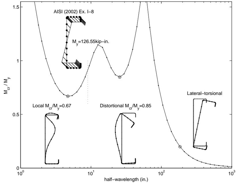
Figure 2 Buckling Modes for a C-section
