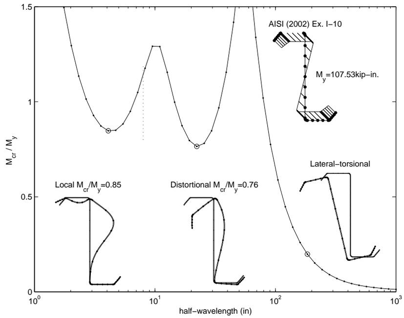
Figure 1 Buckling Modes for a Z-section
