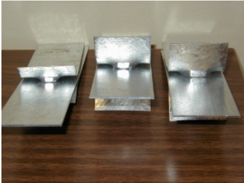
Figure 9: Failed Double Shear Specimens Without Washers
