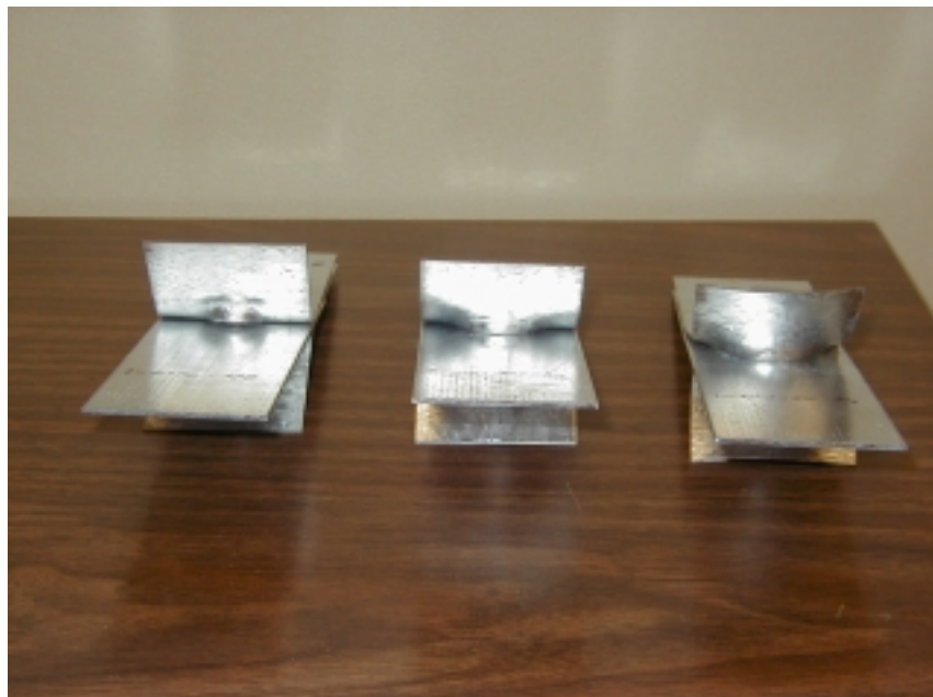
Figure 10: Failed Double Shear Specimens With Washers
