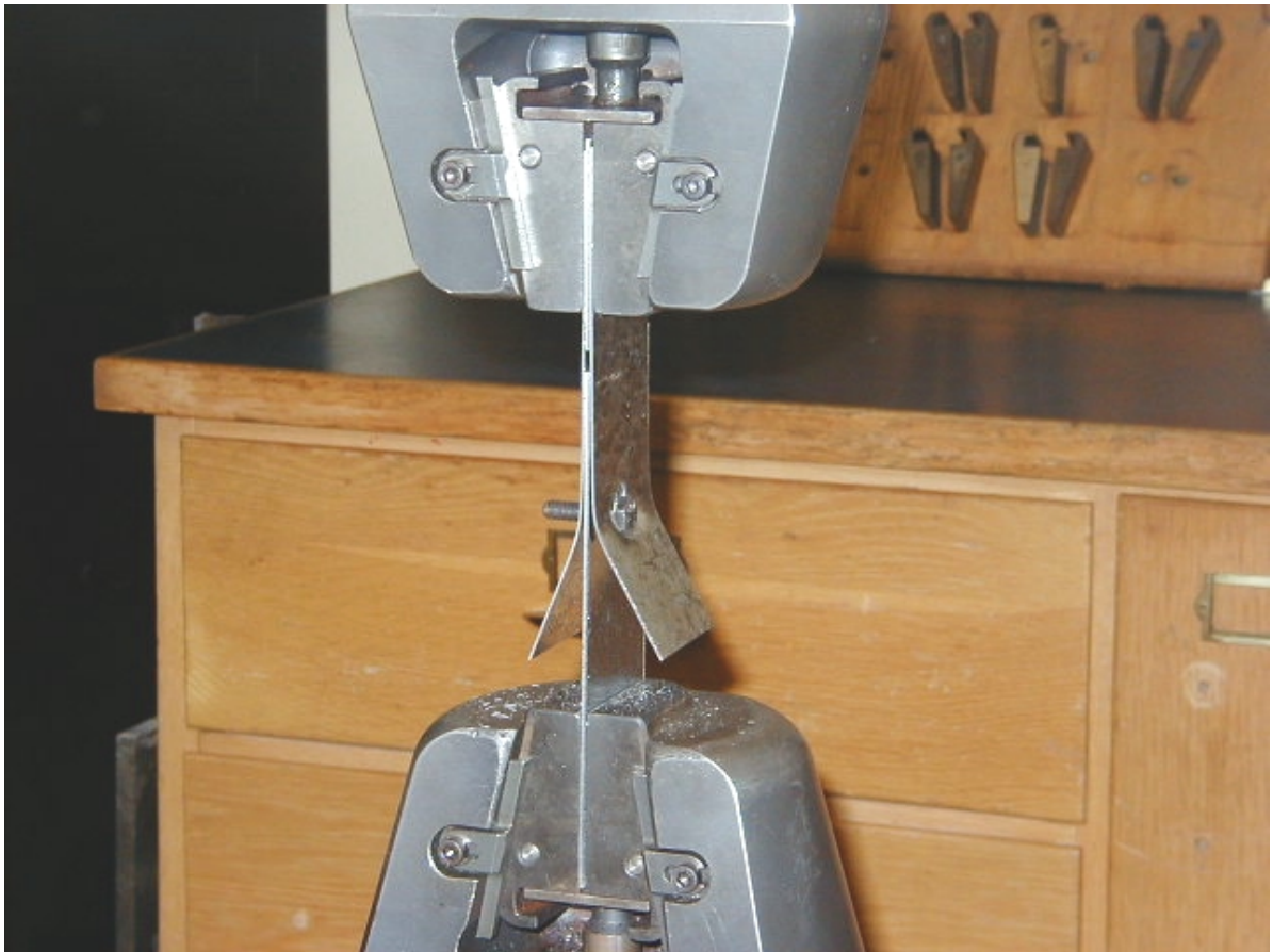
Figure 4: Double Shear Specimen Positioned in Test Frame
