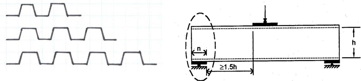
Figure 16 – End One-Flange Loading of Multi-Web Section Specimens
