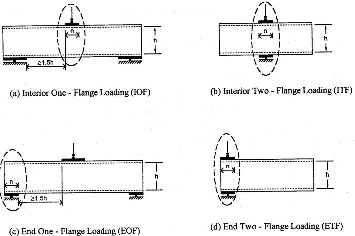
Figure 2 – Load Cases for Web Crippling Tests
