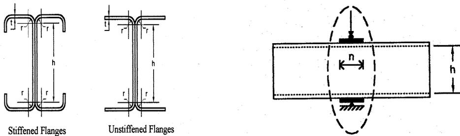
**Figure 5 – Interior Two-Flange Loading of I-Section Specimens**
