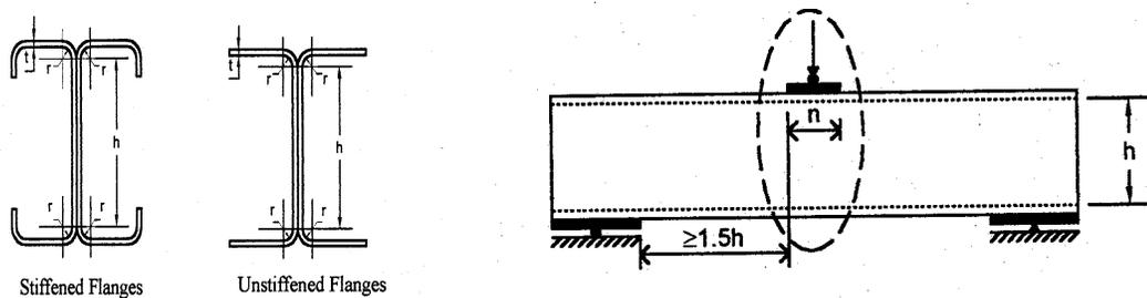
**Figure 3 – Interior One-Flange Loading of I-Section Specimens**
