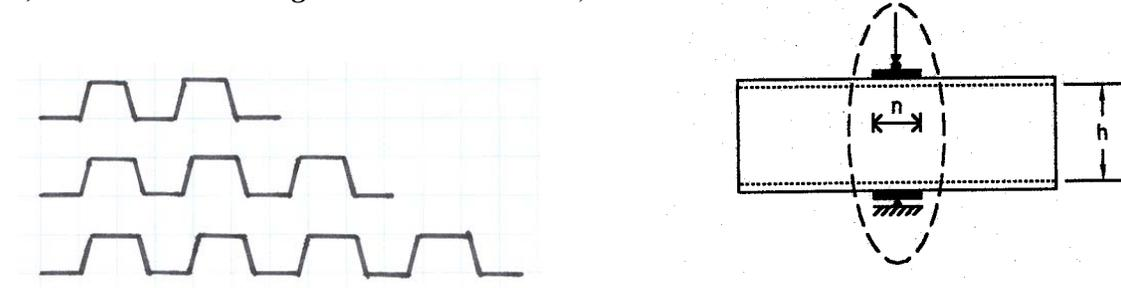
Figure 17 – Interior Two-Flange Loading of Multi-Web Section Specimens
