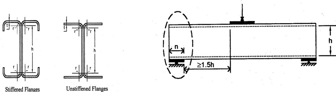
**Figure 4 – End One-Flange Loading of I-Section Specimens**
