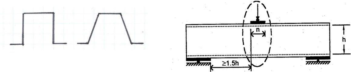
Figure 11 – Interior One-Flange Loading of Single Hat-Section Specimens
