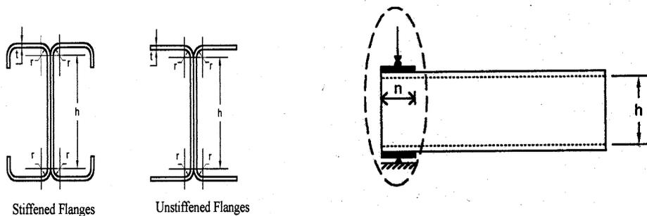
**Figure 6 – End Two-Flange Loading of I-Section Specimens**
