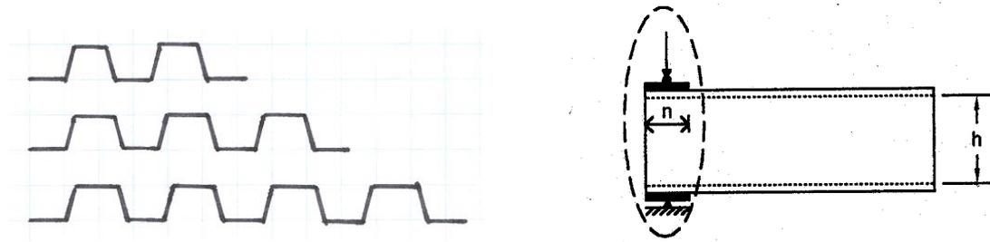
**Figure 18 – End Two-Flange Loading of Multi-Web Section Specimens**
