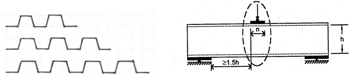
Figure 15 – Interior One-Flange Loading of Multi-Web Section Specimens
