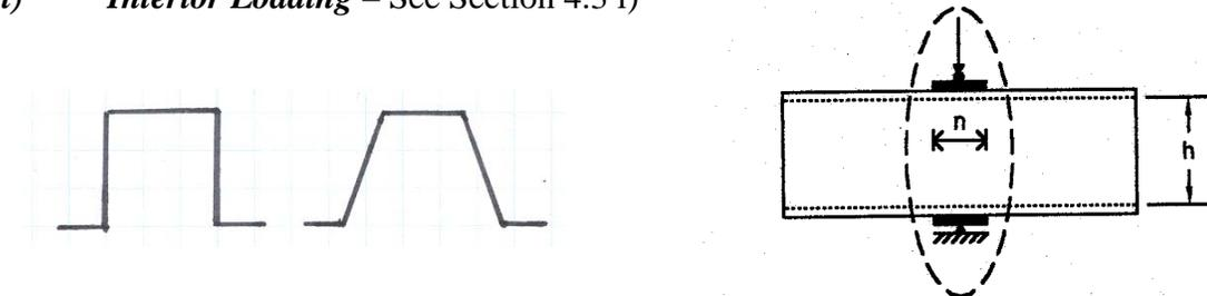
Figure 13 – Interior Two-Flange Loading of Single-Hat Section Specimens
