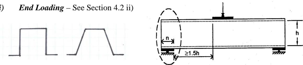
Figure 12 – End One-Flange Loading of Single Hat-Section Specimens
