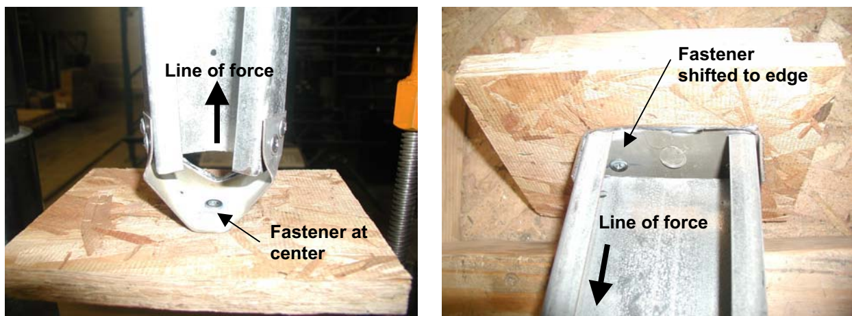
FIGURE 15 FASTENER LOCATIONS FOR STEEL-TO-WOOD WITHDRAWAL TESTS
