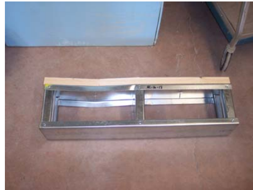
Figure 4.10 – Preferential Span Deflection, Specimen 2C24-18
