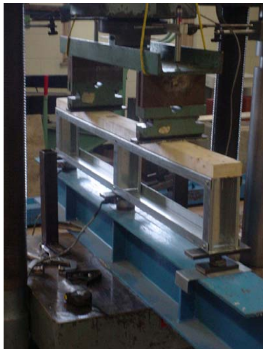
Figure 3.2 – Typical Test Setup of 24 Inch Specimen
