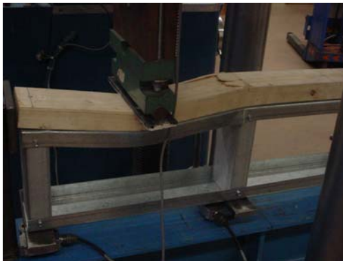
Figure 4.1 – Failed specimen, Group A16-16
