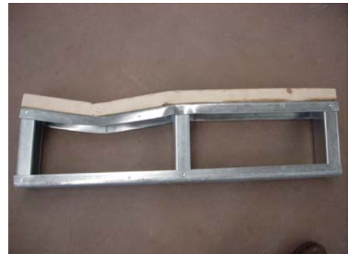
Figure 4.2 – Flexural failure of Specimen 1A16-18
