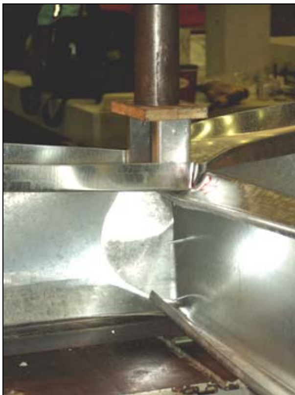
Figure 5.2: Photograph of Excessive Deformation
