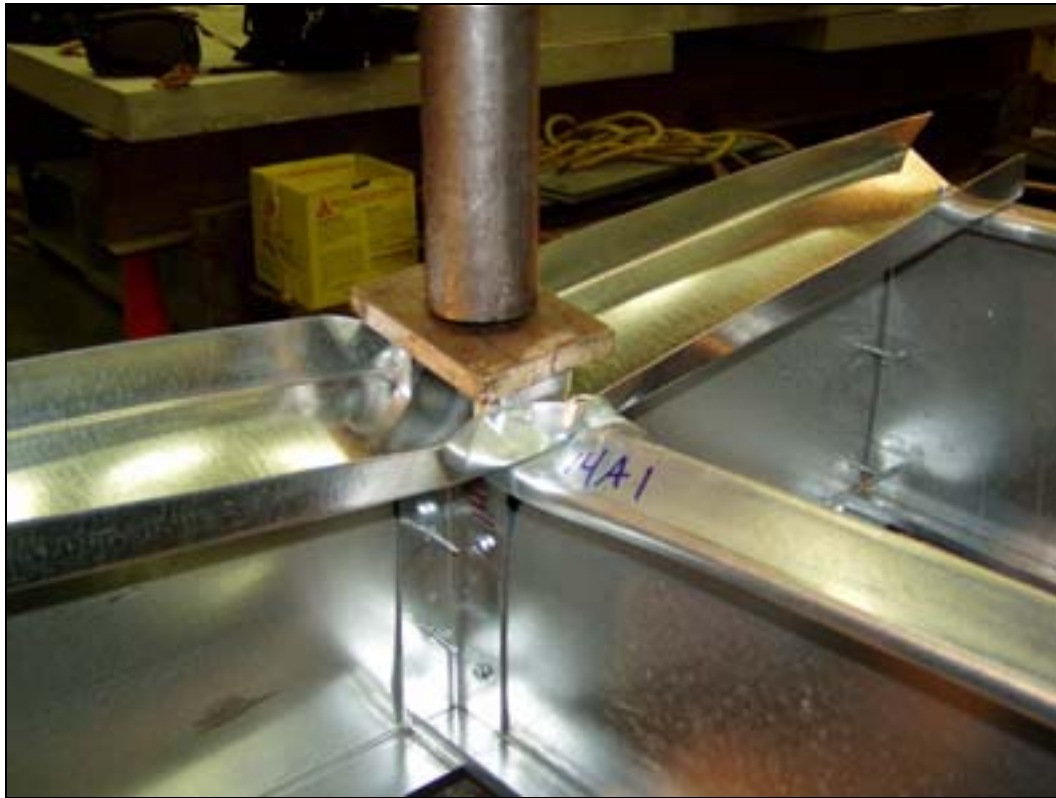
Figure 6.2 Tilting of Loadbearing Stud
