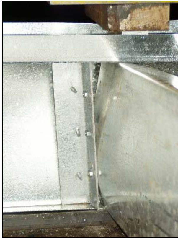
Figure 5.3: Photograph of Screw Shear without Clip Angle Failure
