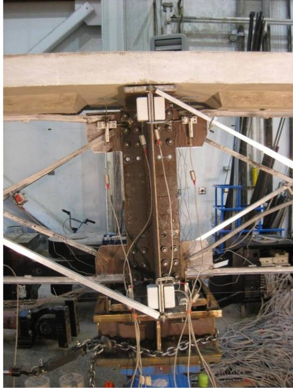
Figure 1-128. Specimen F1B\_1: Middle girder rotation at 5% drift
