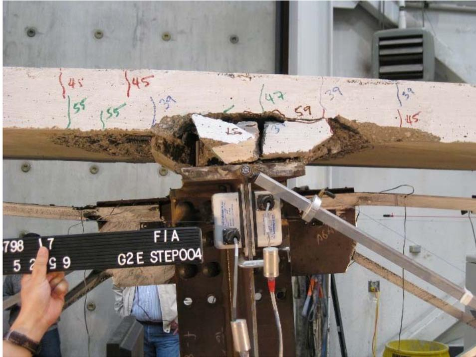
Figure 1-84. FIA Specimen, studded deck to girder connection over Girder 2 at 7.5% drift
