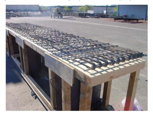
Figure 1-67. Rebar arrangement for Specimen F1C 91
