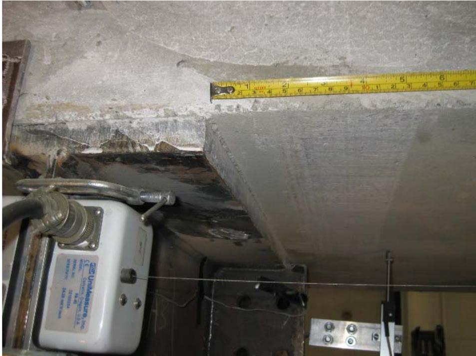
Figure 1-151. Specimen F1C: abrasion of underside of deck shows sliding of the deck
