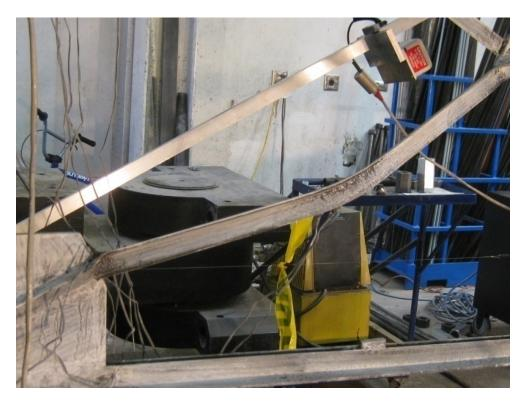
Figure 1-124. Specimen F1B\_1: X-Frame deforming near gusset plate at 3% drift
