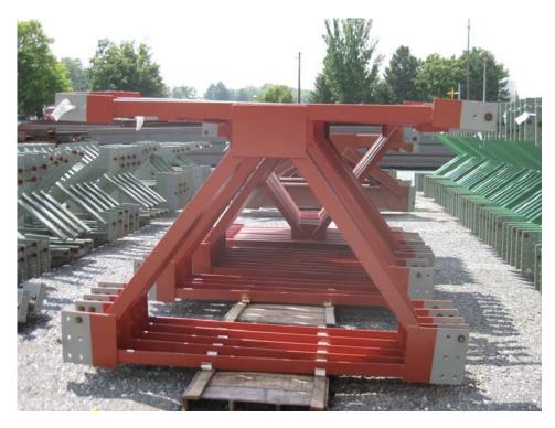
Figure 1-9. Bent cross frames with V-pattern diagonals
