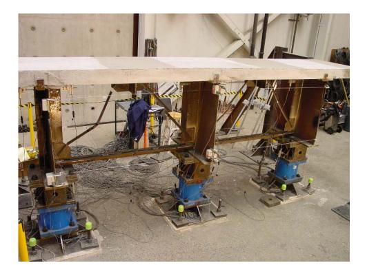
Figure 1-154. Specimen F1C: no damage in the concrete deck after the test
