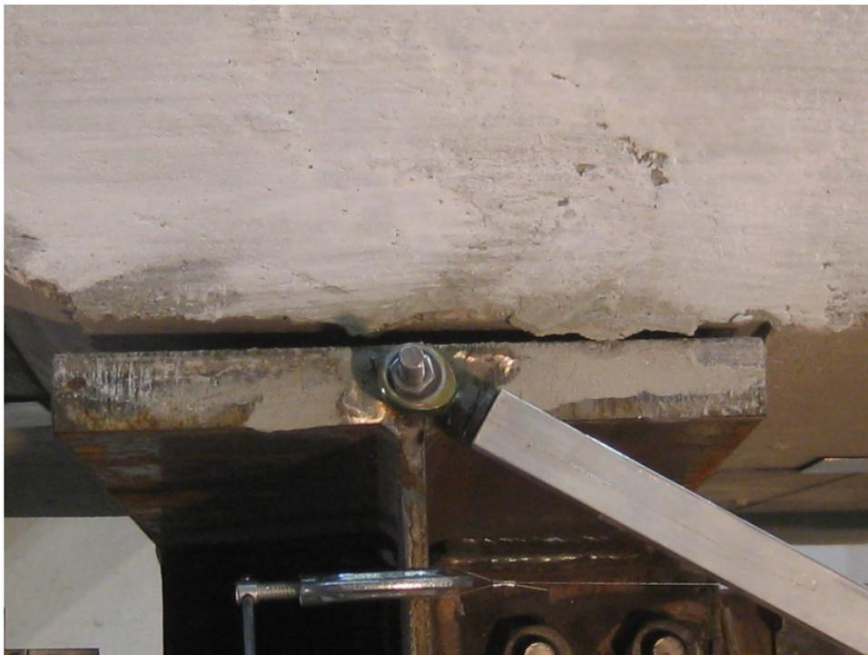
Figure 1-125. Specimen F1B\_1: deck and girder separation at 3% drift
