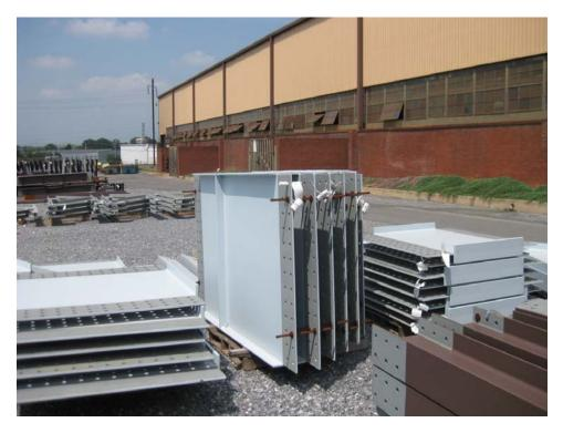
Figure 1-13. Built up I-section diaphragm with transverse stiffener
