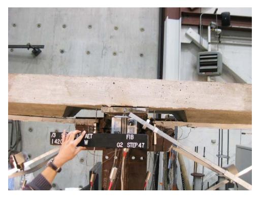
Figure 1-104. Specimen F1B: relative deformation between top chord and deck at 2% drift
