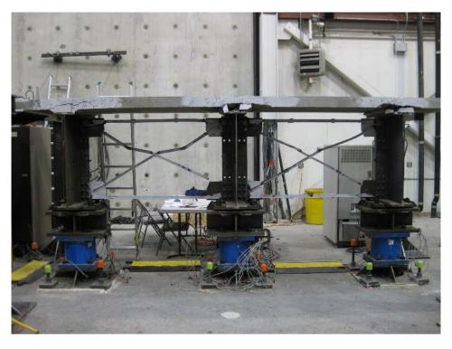
Figure 1-88. Specimen F1A: final damage state at zero displacement
