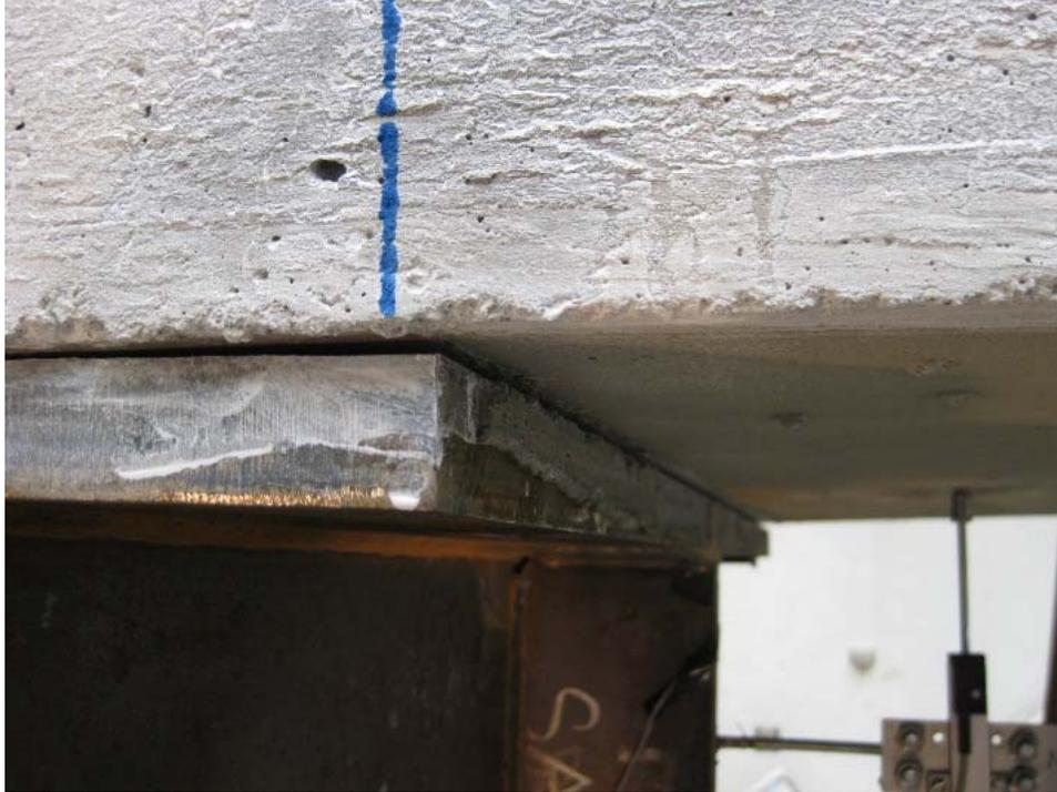
Figure 1-150. Specimen F1C: rotation of the deck over Girder 3 as a result of bending in the deck
