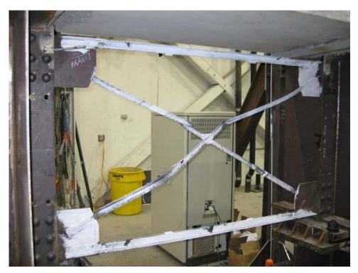
Figure 1-89. Specimen F1A: close-up of cross frame at final damage state at zero displacement
