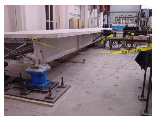
Figure 1-167. Two-girder steel bridge model subjected to reversed static load transverse loading.
