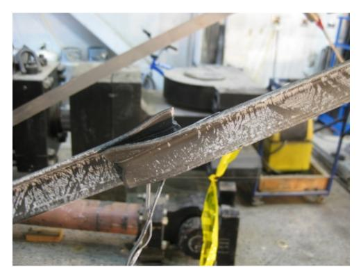
Figure 1-130. Specimen F1B\_1: diagonal failure during 7% drift cycle
