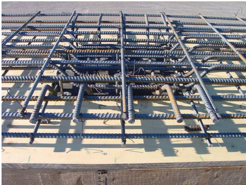
Figure 1-69. Specimen F1C: rebar detail near shear connectors
