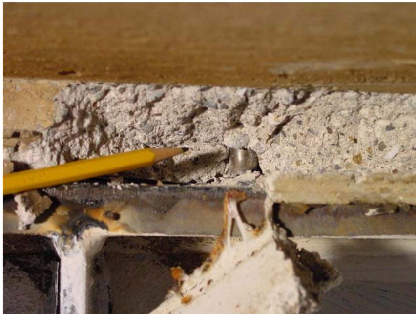
Figure 1-8. Failure of Shear Connectors in Bridge Model during Transverse Cyclic Loading.
