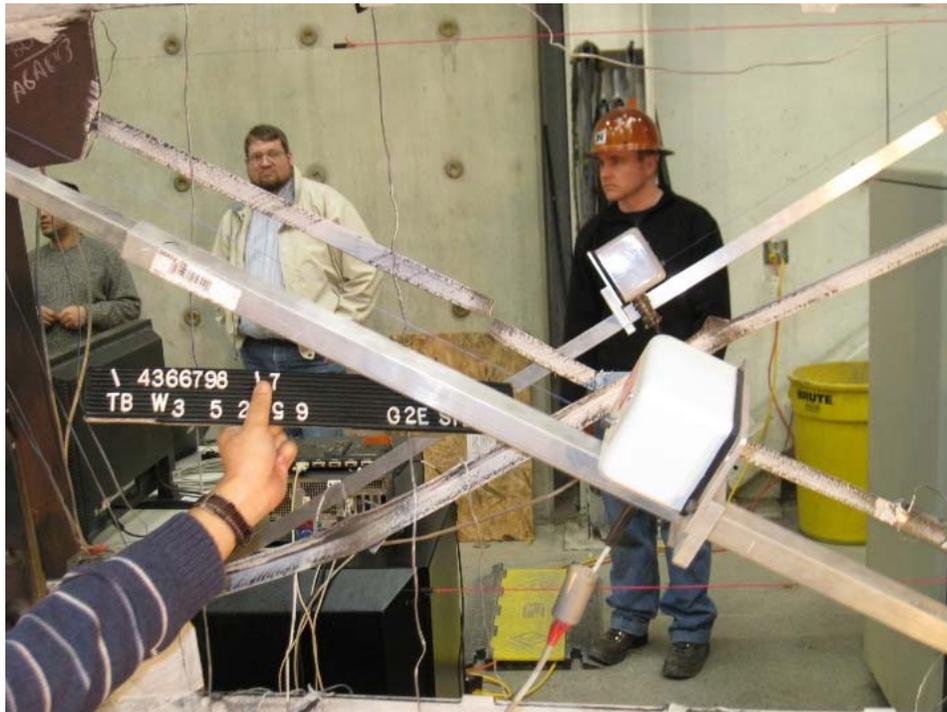
Figure 1-87. View of Specimen F1A at 7.5% drift
