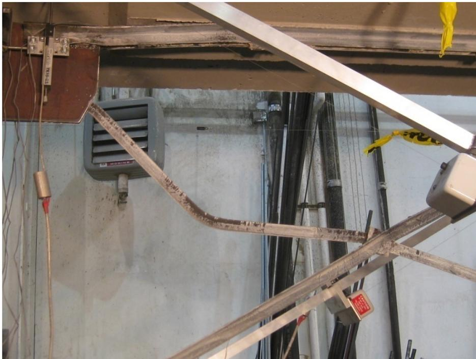
Figure 1-127. Specimen F1B\_1: deformations at 4% drift
