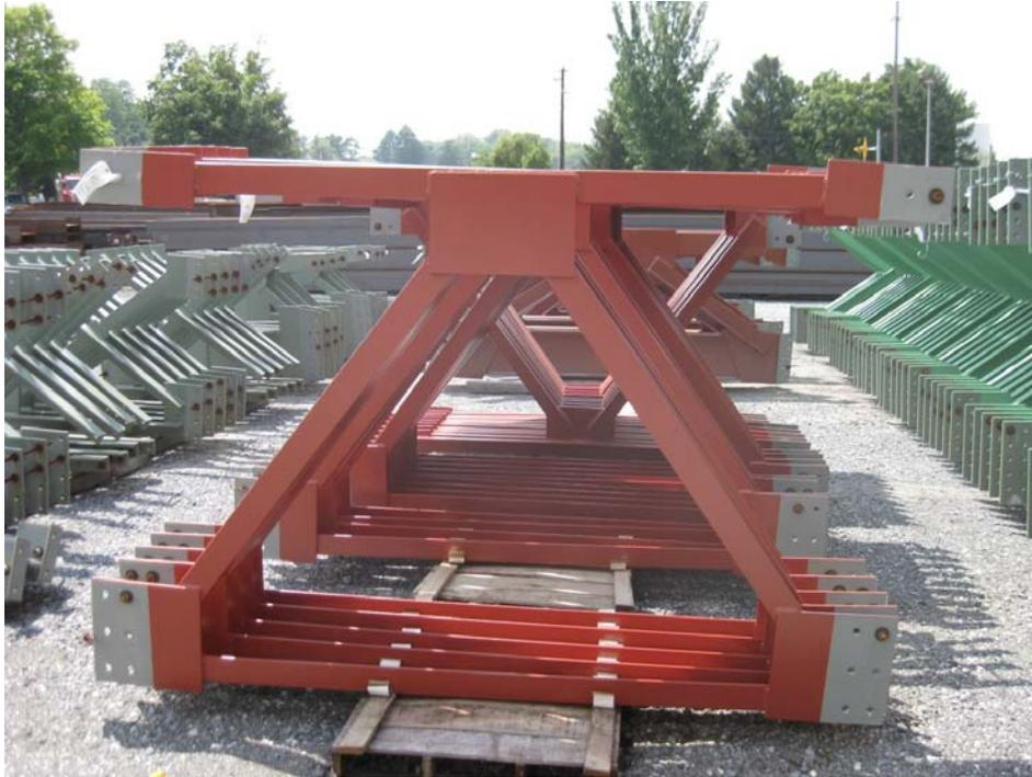
Figure 1-9. Bent cross frames with V-pattern diagonals
