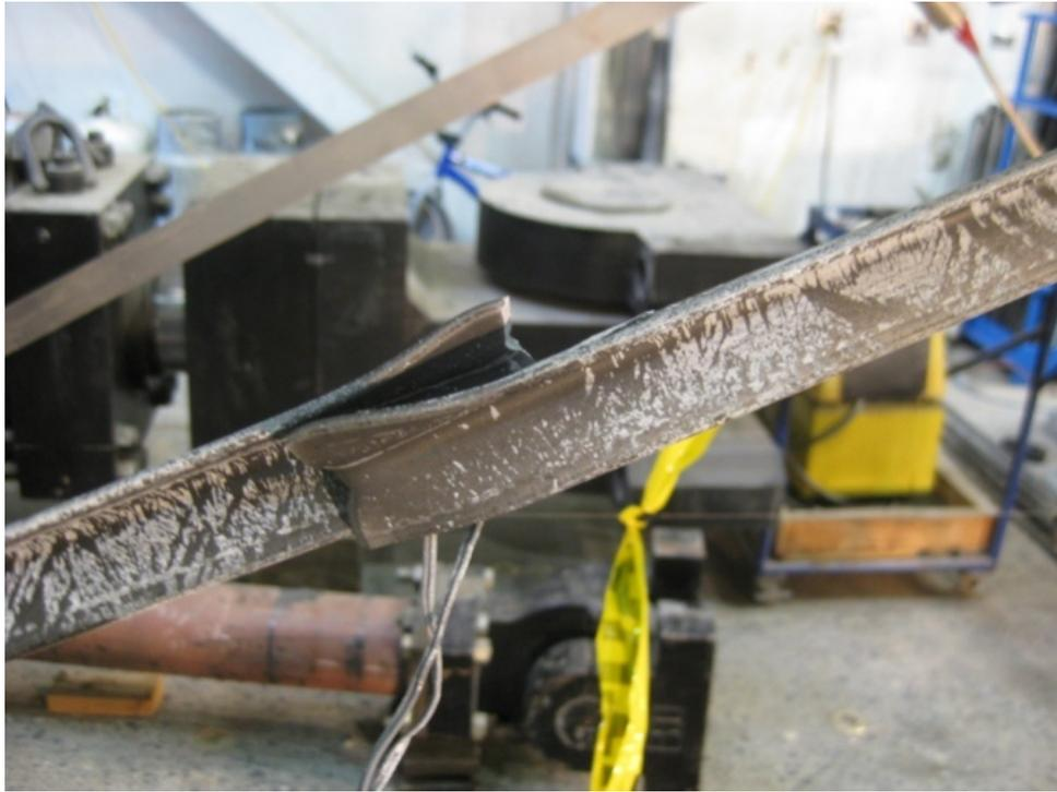
Figure 1-130. Specimen F1B\_1: diagonal failure during 7% drift cycle
