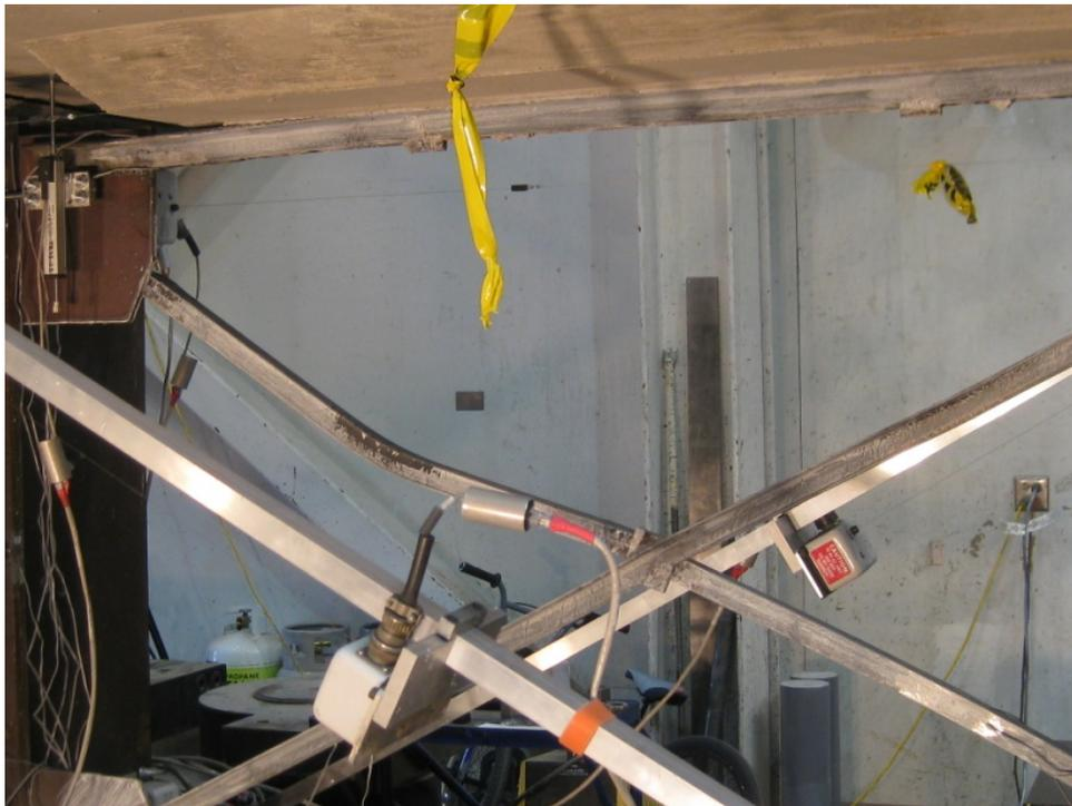
Figure 1-123. Specimen F1B\_1: X-Frame yielding at 2% drift, top chord shows signs of yielding
