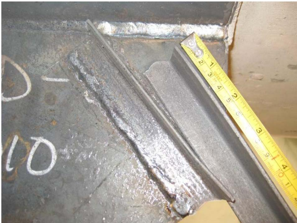
Figure 1-153. Specimen F1C: large permanent axial deformations was observed in braces
