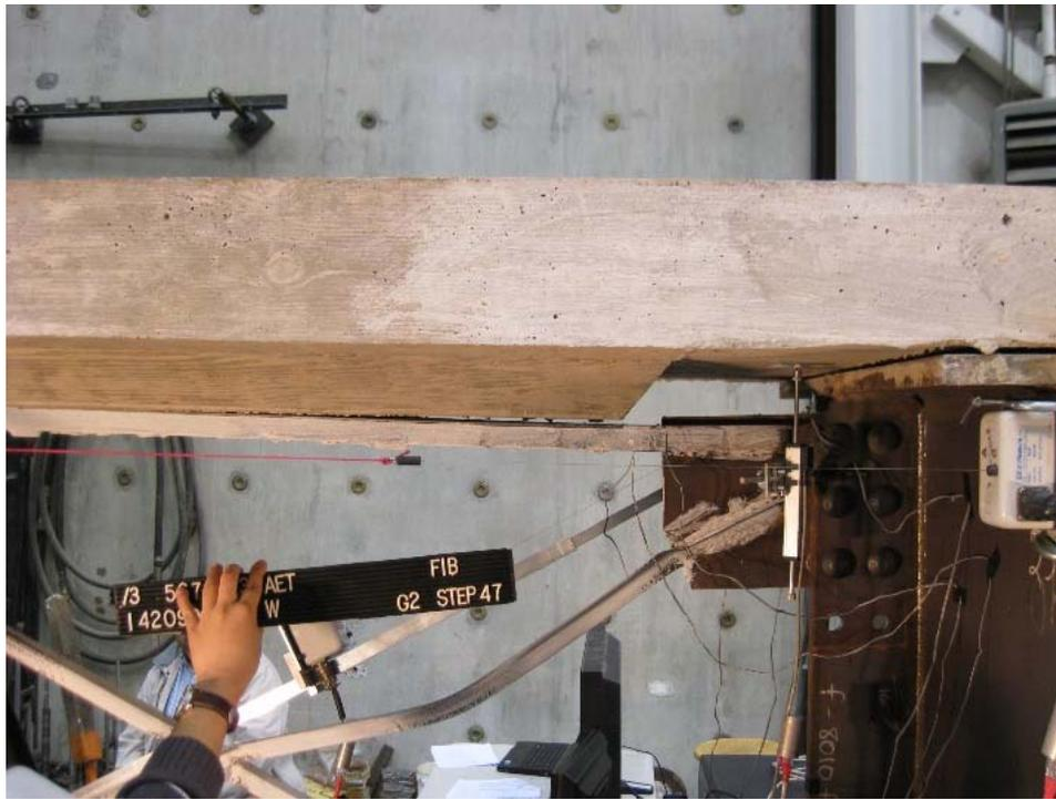
Figure 1-103. Specimen F1B: relative deformation between top chord and deck at 2% drift
