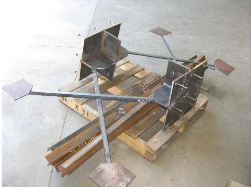
Figure 1-66. Fabricated chevron bracing components before assembly in Specimen F1C
