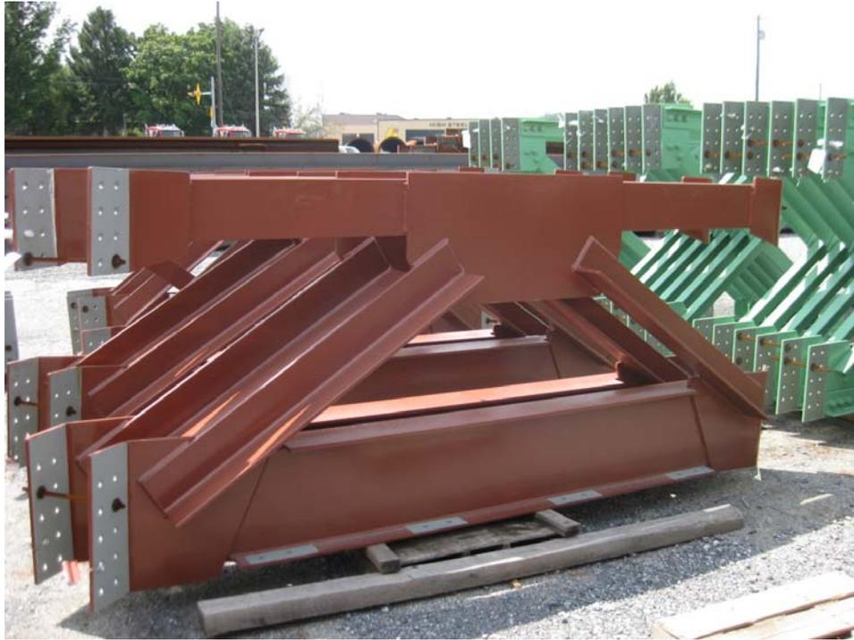
Figure 1-11. Abutment cross frames with V-pattern diagonals
