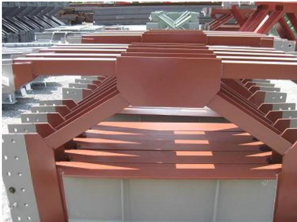
Figure 1-12. Abutment cross frames with V-pattern diagonals
