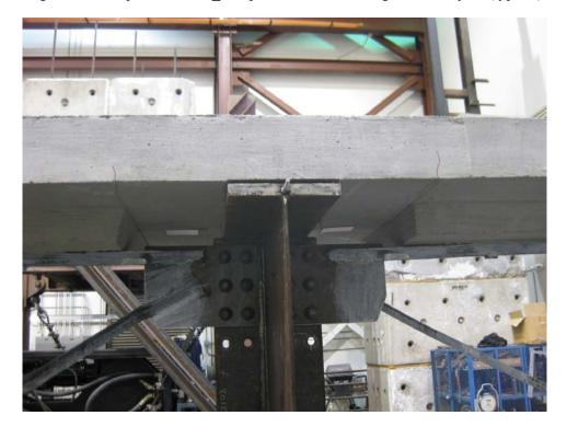
Figure 1-133. Specimen F1B\_1: deck cracks and permanent deck-girder separation - final state
