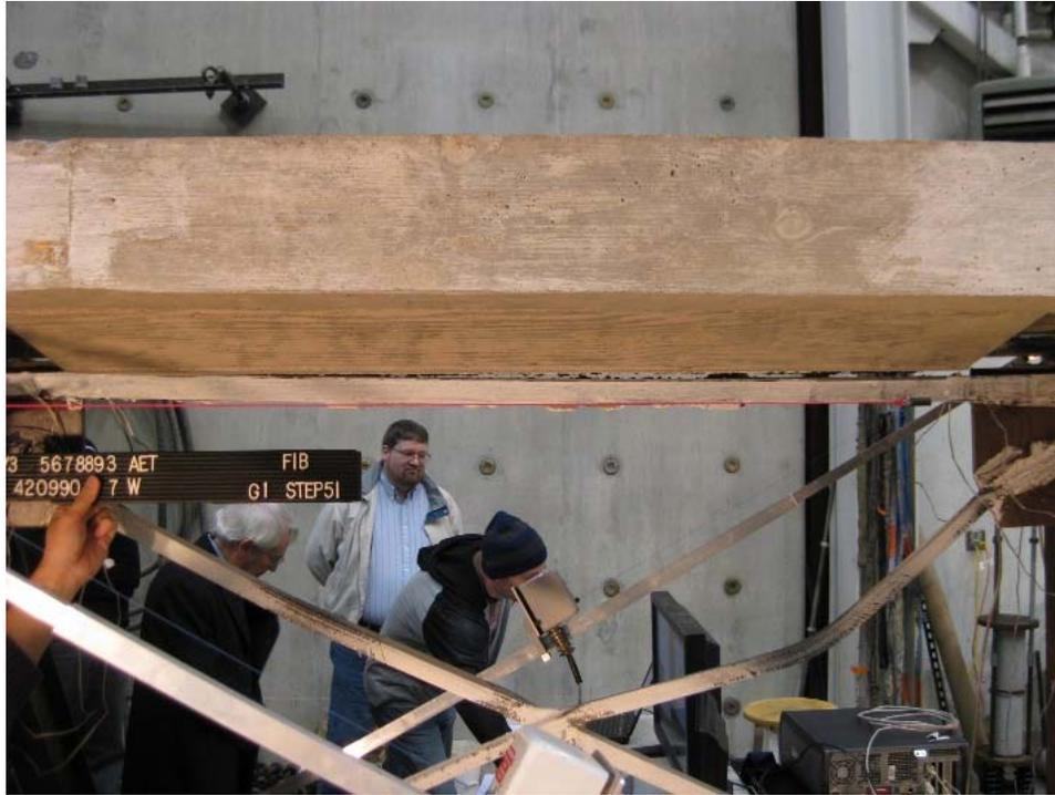
Figure 1-106. Specimen F1B: separation of top chord and deck at 2.5% drift
