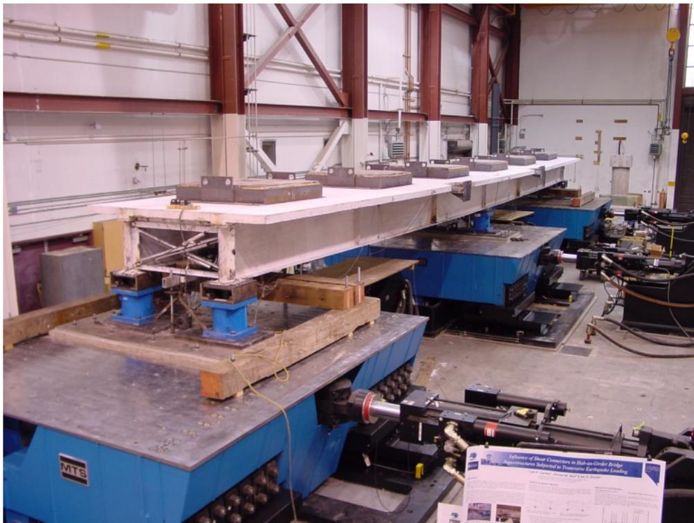
Figure 1-168. Bridge model during shake table experiments with X-braces at the ends.
