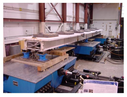
Figure 1-168. Bridge model during shake table experiments with X-braces at the ends.
