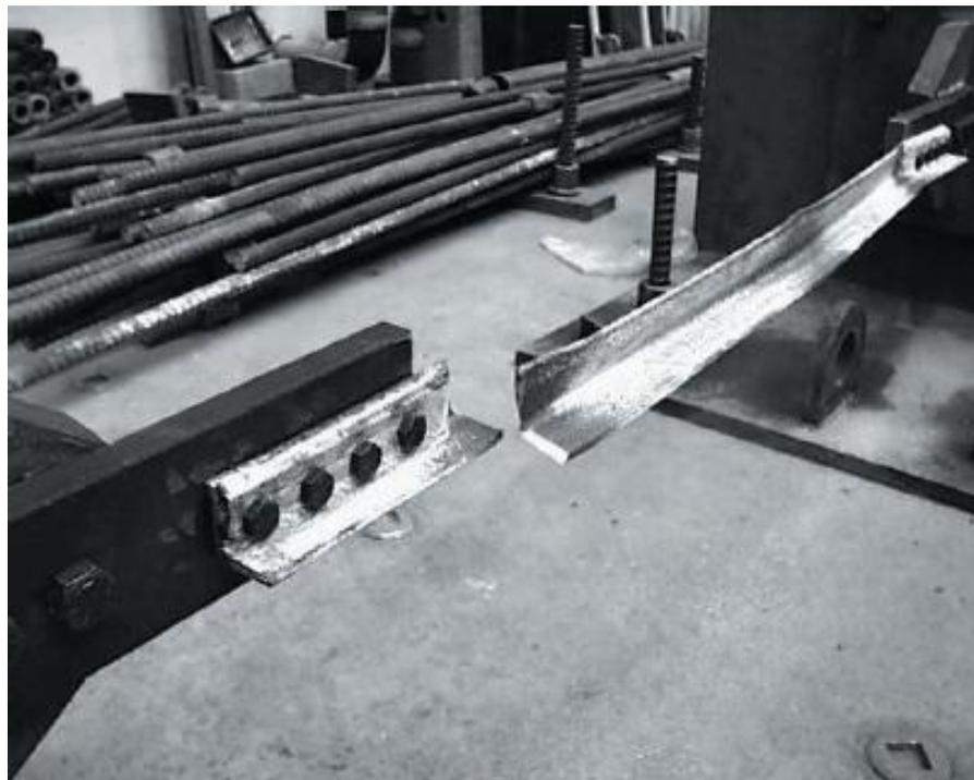
Figure 1-47. Fracture of single angle specimen with thickened bolted connection
