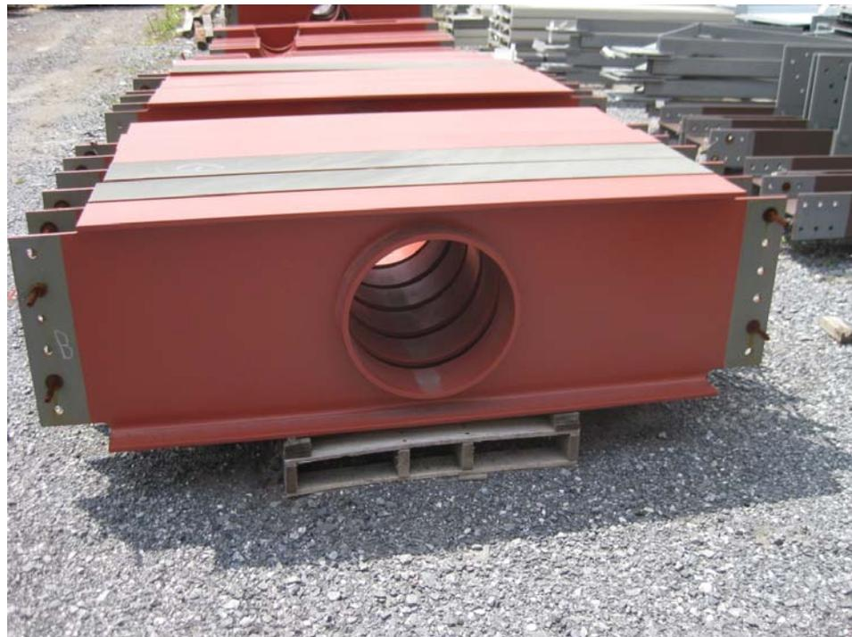
Figure 1-14. Rolled shape diaphragm
