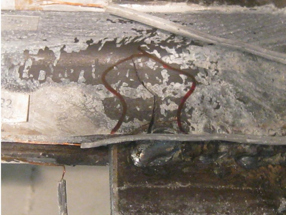
Figure 1-132. Specimen F1B\_1: top chord failure during 7% drift cycle (typical)
