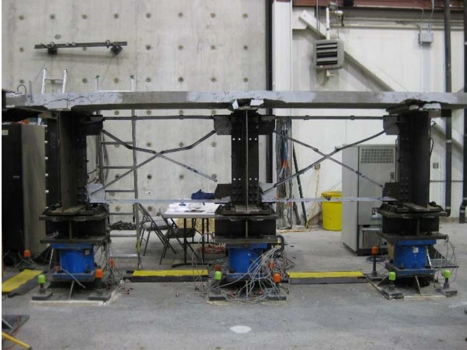
Figure 1-88. Specimen F1A: final damage state at zero displacement
