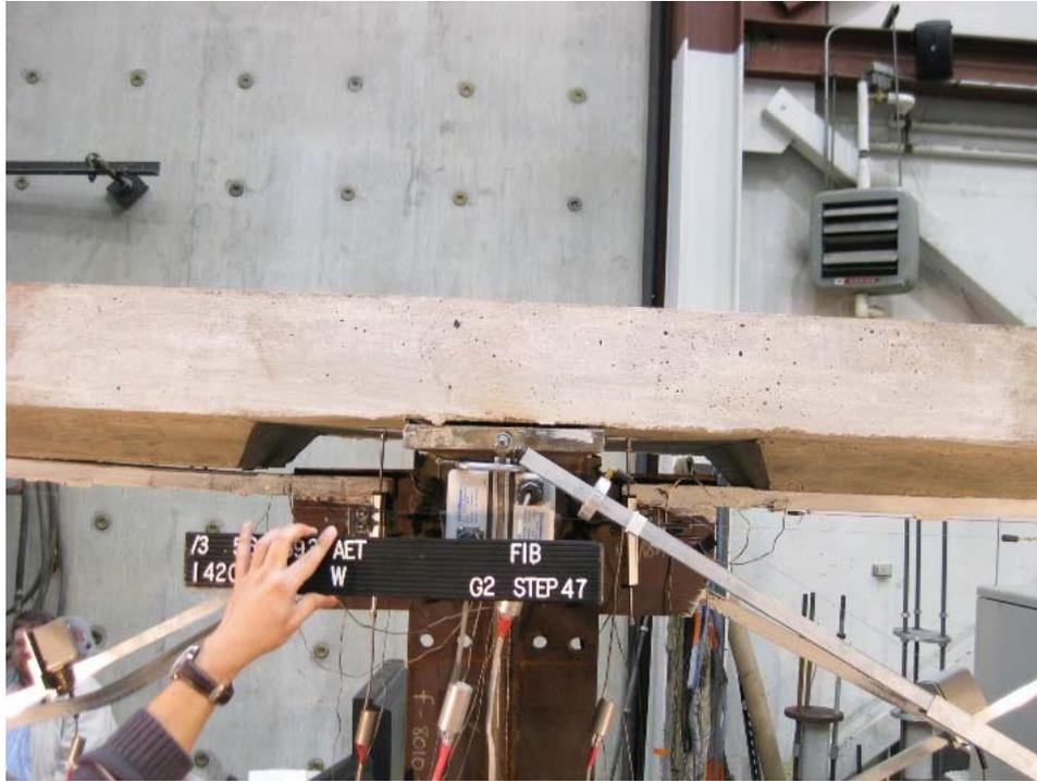
Figure 1-104. Specimen F1B: relative deformation between top chord and deck at 2% drift
