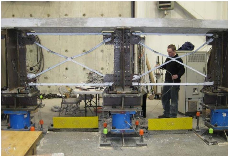
Figure 1-107. F1B Specimen: final damage state at zero displacement
