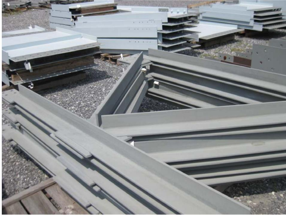
Figure 1-15. Details of cross frames with inverted V-pattern diagonals
