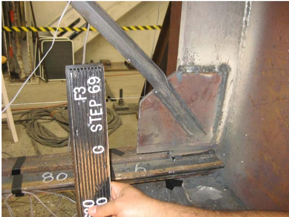
Figure 1-149. Specimen F1C: distortion of buckled angle bracing near the gusset at 2% drift
