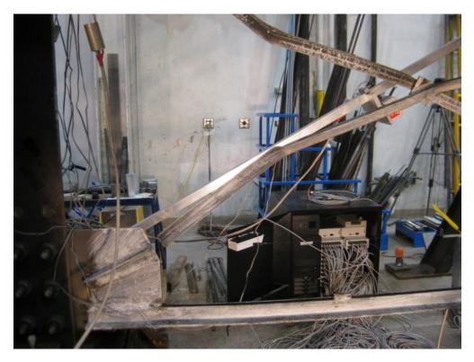
Figure 1-131. Specimen F1B\_1: diagonal failure during 7% drift cycle
