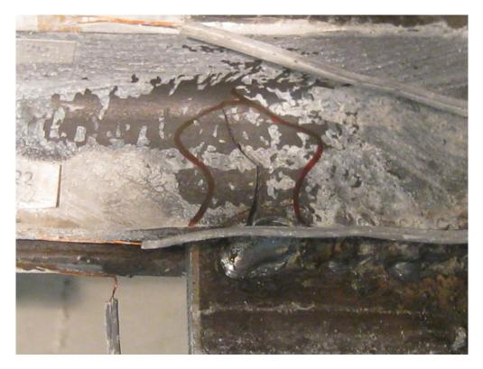
Figure 1-132. Specimen F1B\_1: top chord failure during 7% drift cycle (typical)
