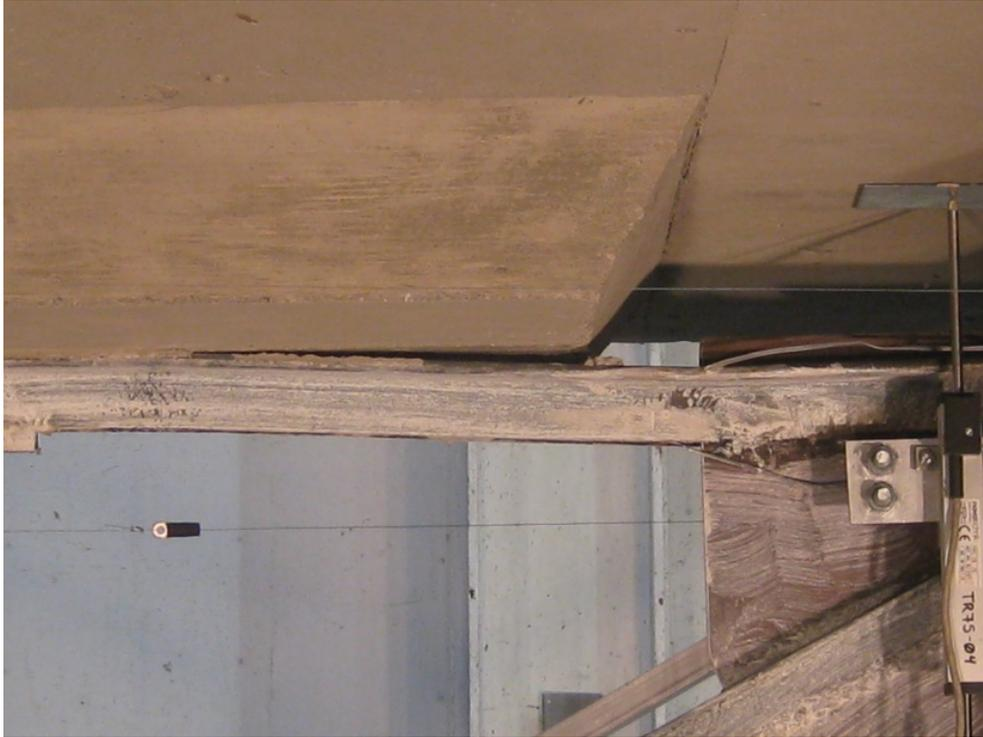
Figure 1-126. Specimen F1B\_1: top chord at 3% drift
