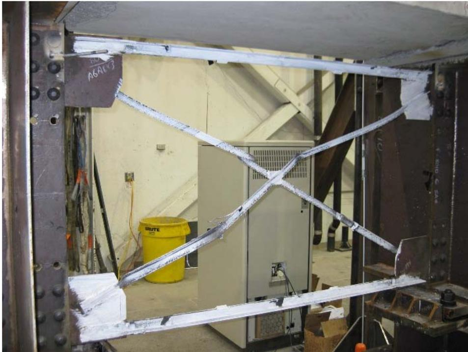
Figure 1-89. Specimen F1A: close-up of cross frame at final damage state at zero displacement
