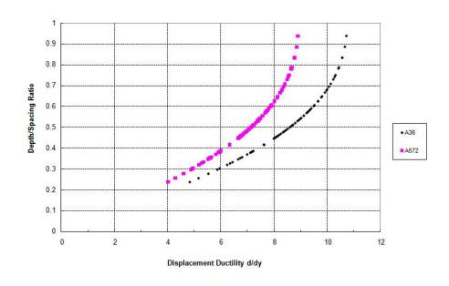
Figure 1-37. Limitation of D/S ratio for 4% drift limit
