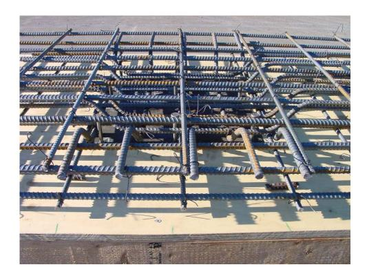
Figure 1-69. Specimen F1C: rebar detail near shear connectors 92
