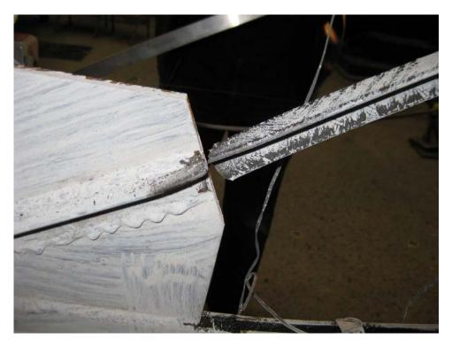
Figure 1-82. F1A Specimen, rupture of one diagonal brace at 5% drift
