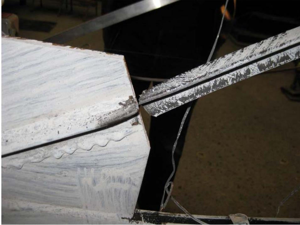
Figure 1-82. F1A Specimen, rupture of one diagonal brace at 5% drift
