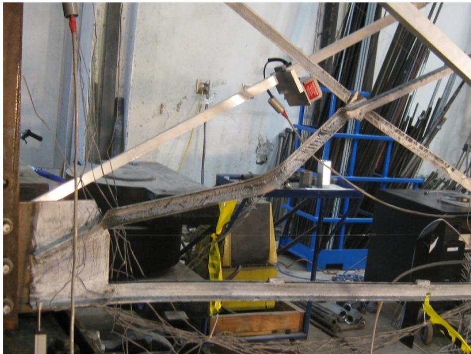
Figure 1-129. Specimen F1B\_1: deformations at 6% drift
