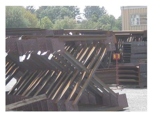
Figure 1-10. Bent cross frames with X-pattern diagonals
