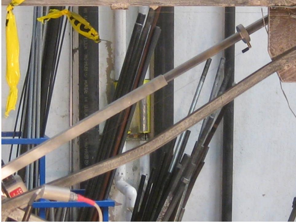
Figure 1-122. Specimen F1B\_1: X-Frame buckling at 1% drift
