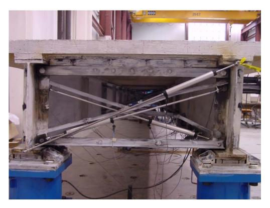
Figure 1-173. South end of bridge model after reversed static load experiment with ductile X-braces.
