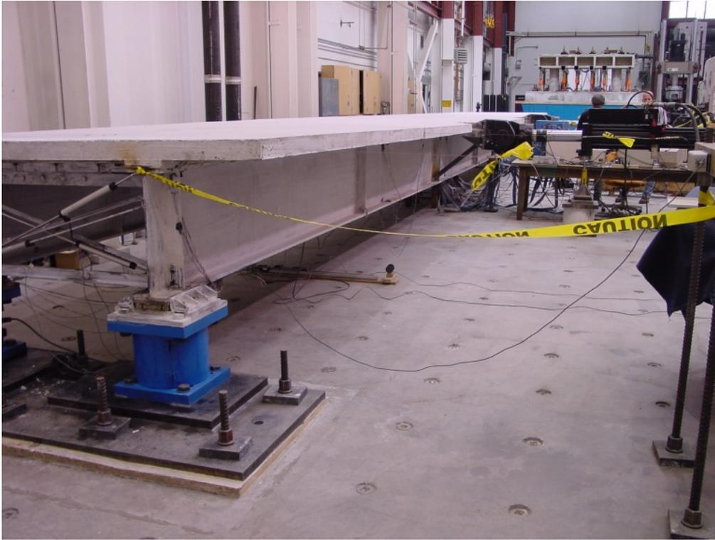
Figure 1-167. Two-girder steel bridge model subjected to reversed static load transverse loading.
