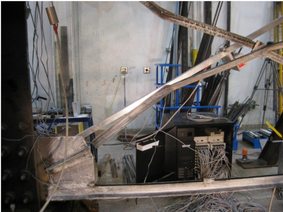
Figure 1-131. Specimen F1B\_1: diagonal failure during 7% drift cycle
