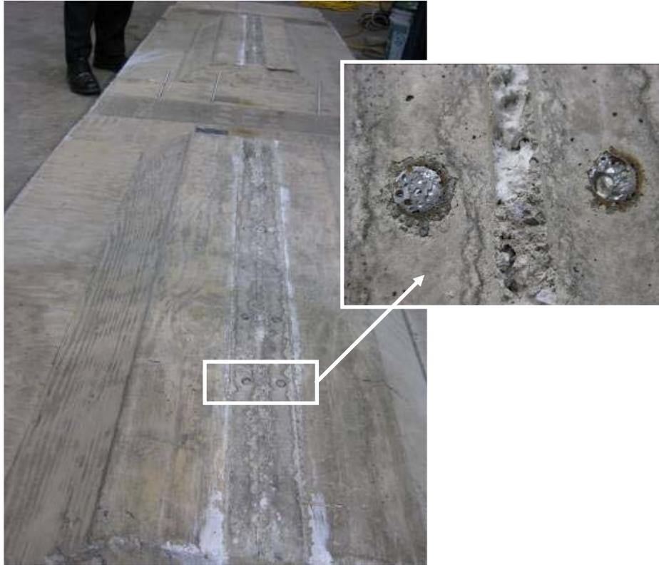
Figure 1-108. F1B Specimen: close-up of underside of deck showing premature failure of stud connections
