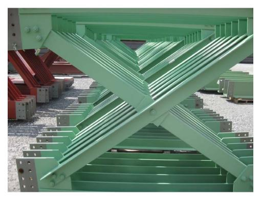
Figure 1-21. Details of cross frames with X-pattern diagonals
