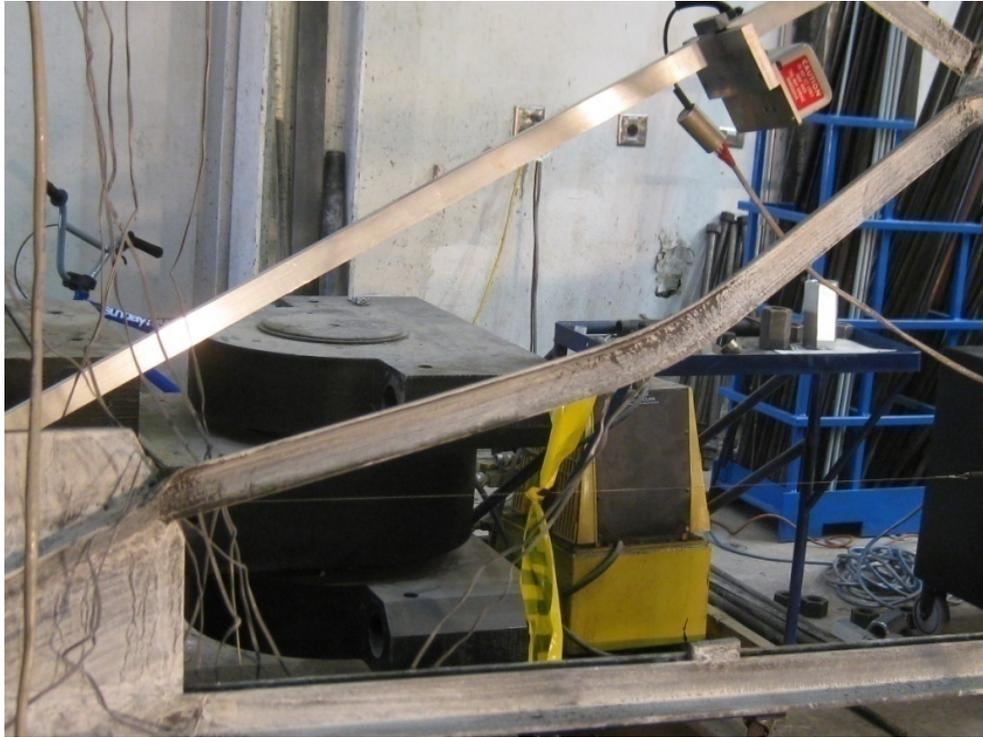
Figure 1-124. Specimen F1B\_1: X-Frame deforming near gusset plate at 3% drift
