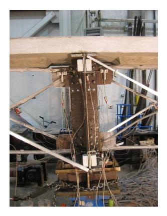
Figure 1-128. Specimen F1B\_1: Middle girder rotation at 5% drift
