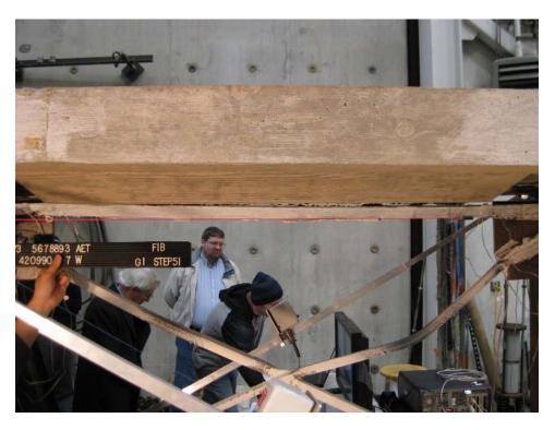
Figure 1-106. Specimen F1B: separation of top chord and deck at 2.5% drift
