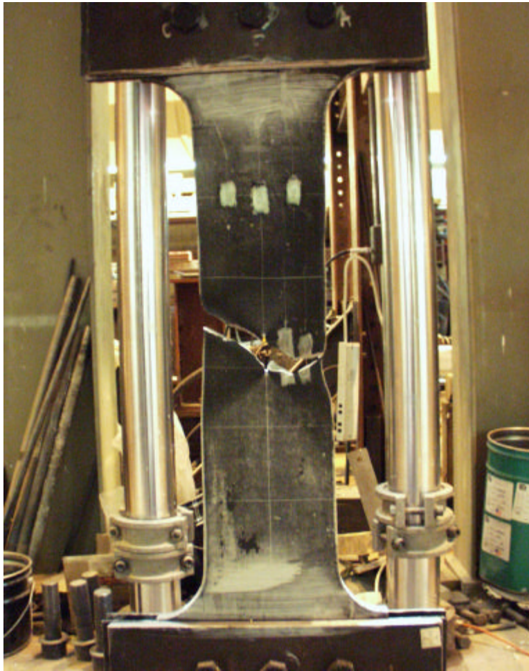
Figure 2.12– Final state of HPS70W-1.1-H specimen
