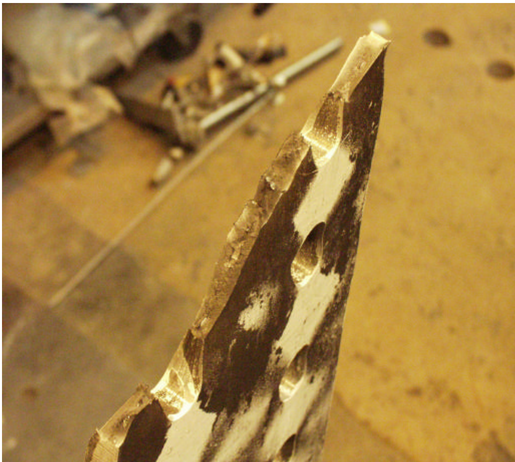
Figure 2.14 – Fracture surface of HPS70W-12h specimen
