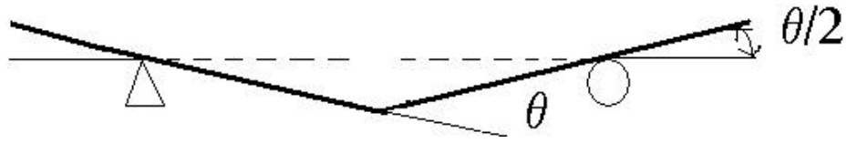
Figure 1.2 – Definition of rotation angles at the end and at the center of a beam
