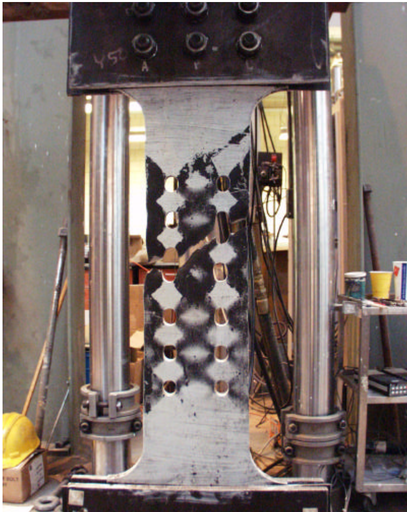
Figure 2.13 –Final state of HPS70W-12h specimen
