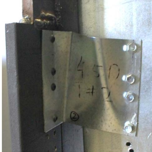
Figure 5.6: Failure mode of shear test II4.5 #b2
