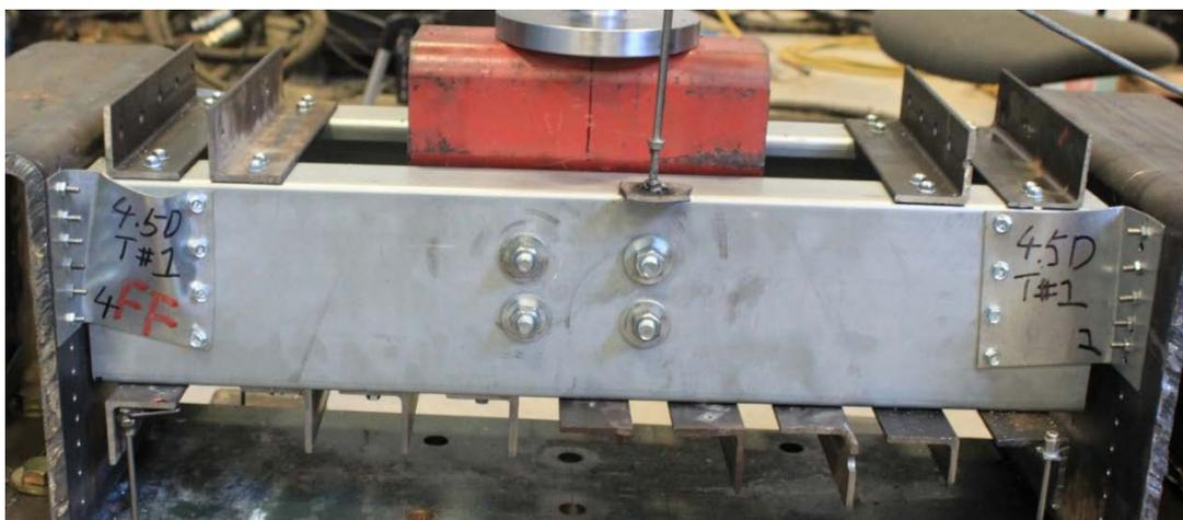
Figure 5.5: Failure mode of joist 4.5D T#1
