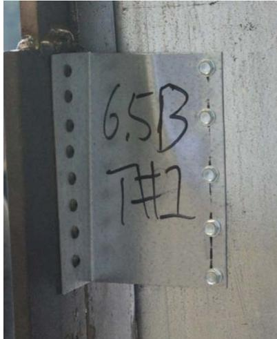
Figure 5.9: Failure mode of shear test II6.5 #1
