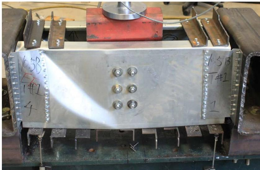
Figure 5.11: Failure mode of Test 10.5B #1
